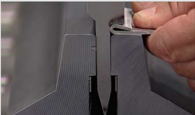
Pre-bend and flattening in the same tool.
